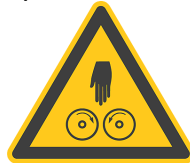
Pinch point Hand in rollers
