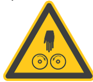
Pinch point Hand in rollers
