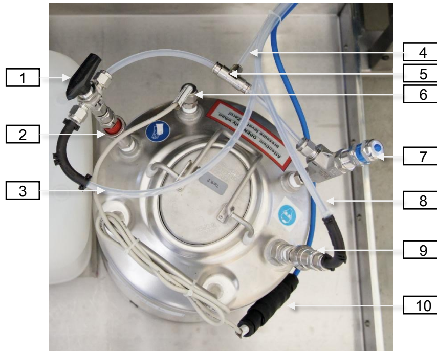
Figure 9: Pressure tank PGMEA
