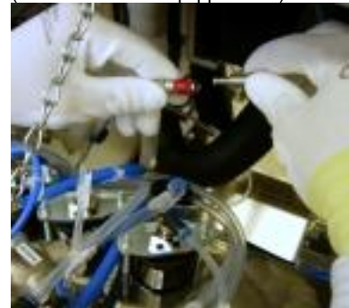
3. Disconnect the BSR quick connector (if the machine is equipped with)
