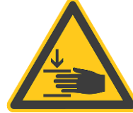
Squeezing hazard Hand crush
